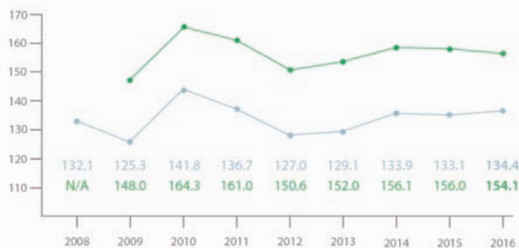
Kilowatt hours of energy used in production as a proportion of production output (kWh/tonne)
